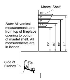
Figure 11 - Minimum Mantel Clearances for Built-In Installation
